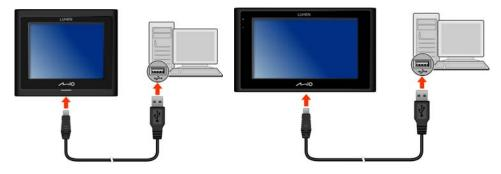
3. The charge indicator glows amber when charging is in progress. When the battery is fully charged, the indicator turns green.
